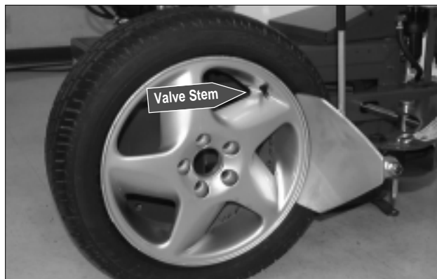
Figure 20 - Position Tire for Bead Loosening
