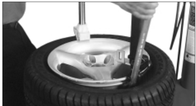
Figure 29 - Rotate Lifting Tool Down for Demount
