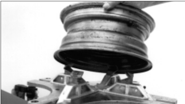
Figure 5 – Place Tire/Wheel Assembly on Table Top
