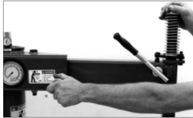
Figure 7 - Adjust Swing Arm to Position Head Roller
