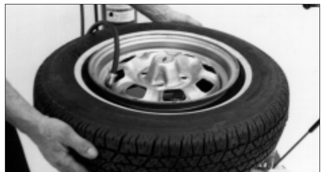
Figure 18 - Lift Tire Upwards for Bead Sealing
