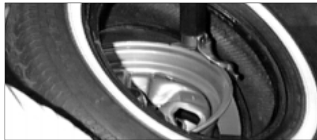
Figure 16 - Position Tire Against Mount/Demount Head
