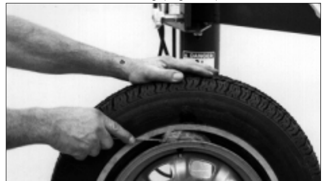
Figure 3 – Apply Rubber Lubricant to Tire Beads
