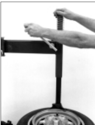
Figure 6 - Position Mount/Demount Tool
