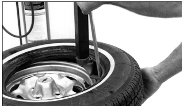
Figure 12 - Demounting Lower Bead
