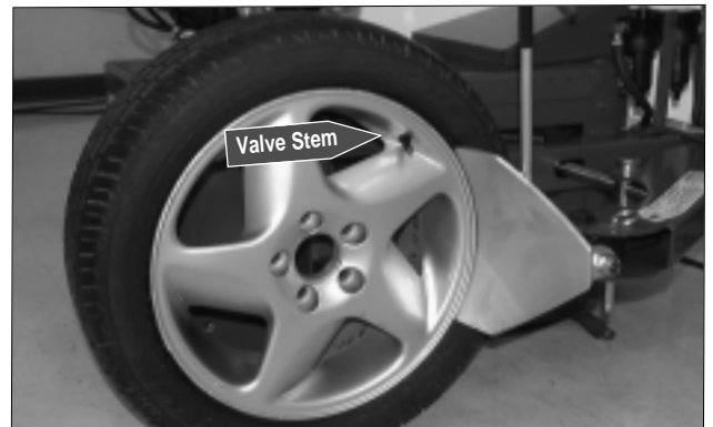
Figure 2 – Position Tire and Bead Loosener Shoe
