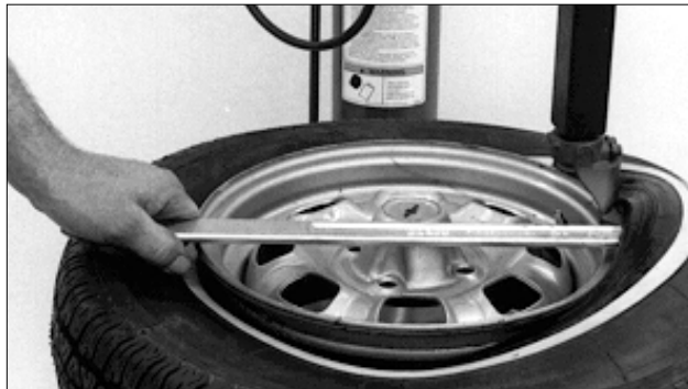
Figure 11 - Lift Bead Over Demount Head
