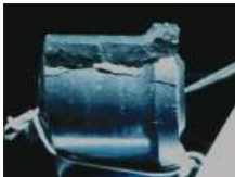
Cracked grommet during ozone test
