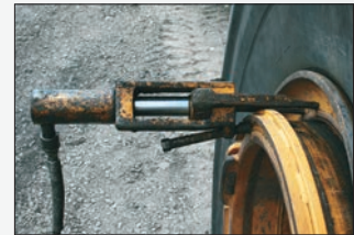
The Giant Tire/Earthmover Tire Bead Breaker in use.
