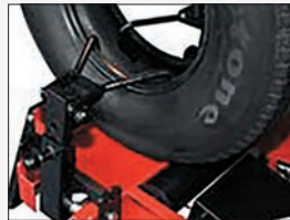
The Automatic Truck Tire Spreader in use.
